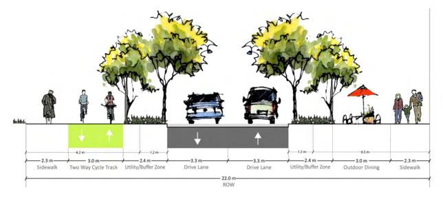
Figure 8.8 Kapyong Minor Collector Street Type B Section with Parking
