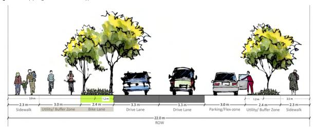
Figure 8.6 Kapyong Minor Collector Type B Street Section
