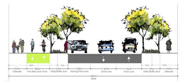
Figure 8.9 Kapyong Minor Collector Street Section with a Bike Share Station
