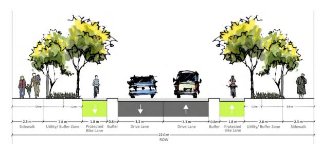
Figure 8.5 Kapyong Minor Collector Type A Street Section
